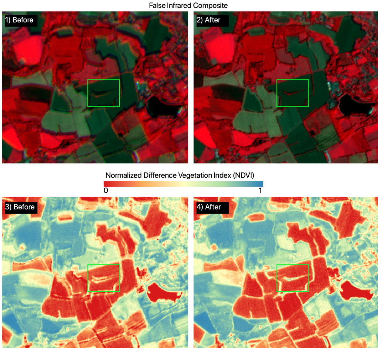
Figure 3: Images 1 and 2 are showing before and after of false infrared composite. Images 3 and 4 show NDVI values. Using the green box as context, notice the edges of healthy vegetation is prominent in image 4 than in image 3.
